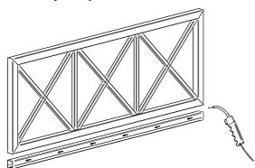
1) Prepare a Guide of length S and weld under the gate.
