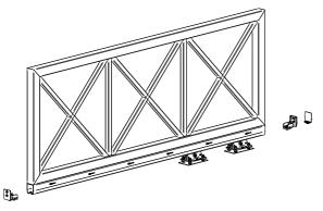
3) Slide the gate guide over the trolleys and fix the Guide Roller on one end and a Guide Roller and/or the Front Cover on the other end.
