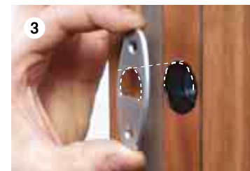
3 Insert the cover tray in the hole, place the striker so as to bring the circular profiles and fix with two screws.
