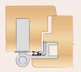
For profiles with gasket on rebate, 10/12 mm
