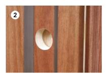
The striker installation has never been so simple: it just takes a milling of ø 25 mm and a drill. Jigs are not required.
